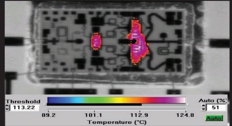
The hot regions on an integrated circuit due to the drive and output transistors
