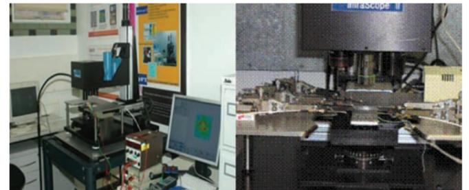
Quantum Focus microscope and micro-probe station
