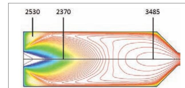
Combustion chamber temperature contours illustrating the flame shape. Image courtesy of Monitor Coatings Ltd and Southampton University
