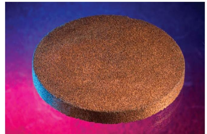
Heat transfer coefficient of porous copper made by the LCS process. The pore size was nominally 700microns
